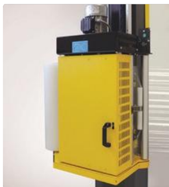
LP - Powered pre-stretch 240% (150%-200% - kit available as option)
