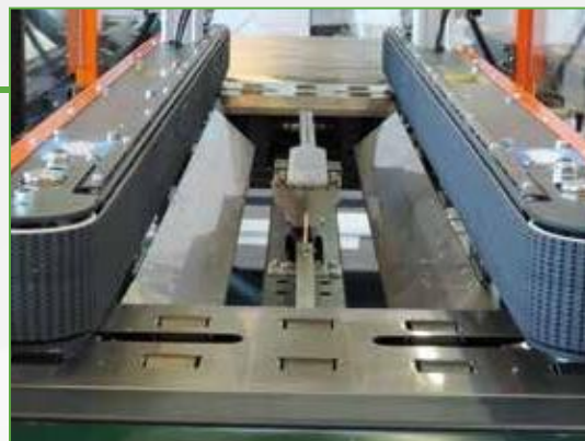
Folding system of bottom flaps (only HM11-TB)
